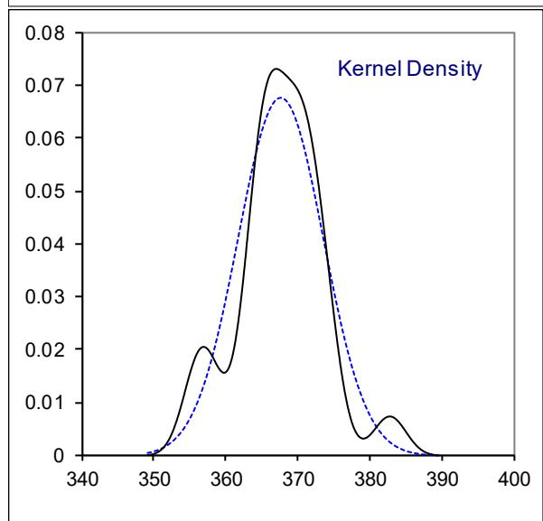
Determination of Viscosity Stabinger at 100°C on sample #20095; results in mm<sup>2</sup>/s
