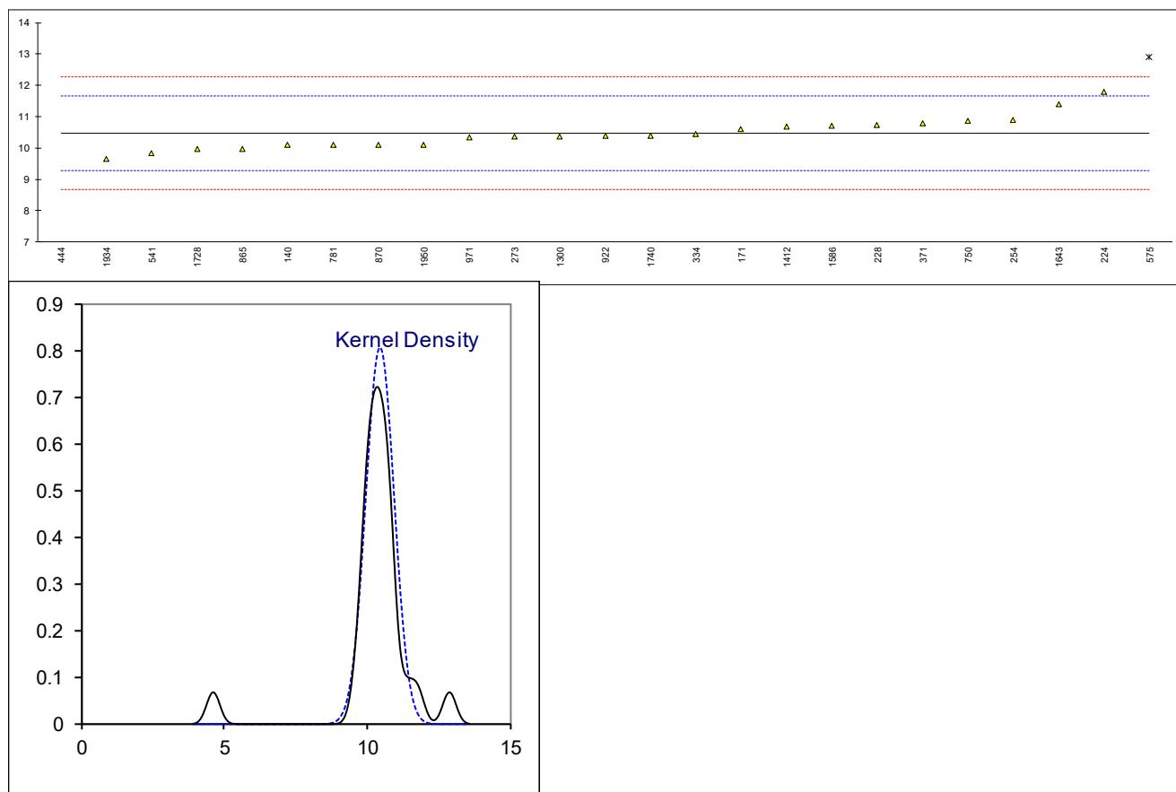
Determination of Density at 15°C on sample #20095; results in kg/m<sup>3</sup>
