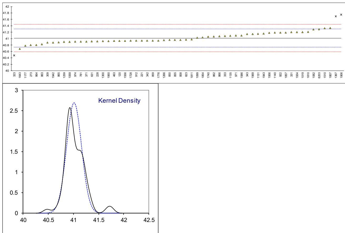
Determination of Kinematic Viscosity at 50°C on sample #20095; results in mm<sup>2</sup>/s
