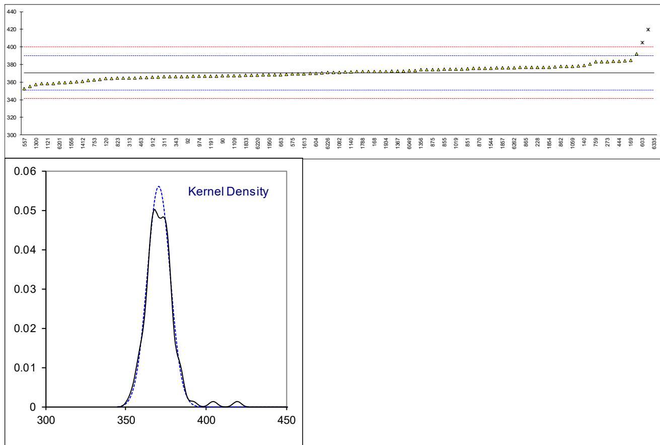
Determination of Kinematic Viscosity at 100°C on sample #20095; results in mm<sup>2</sup>/s
