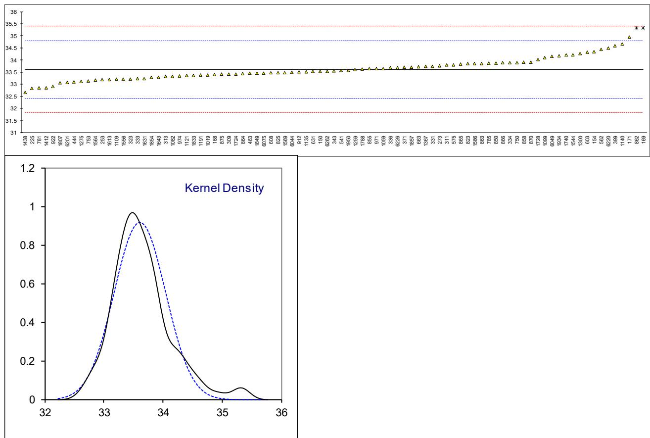
Determination of Viscosity Stabinger at 50°C on sample #20095; results in mm<sup>2</sup>/s
